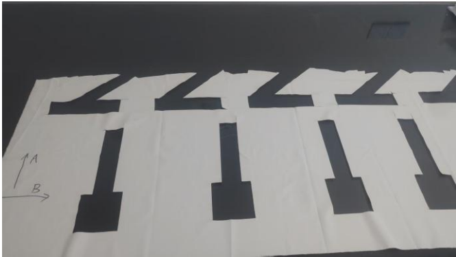
PG1 at the test lab, specimens cut out; A and B mark the two test directions. Cream, as supplied.
