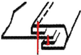
BSg 3.14.01 · binding, two operations
